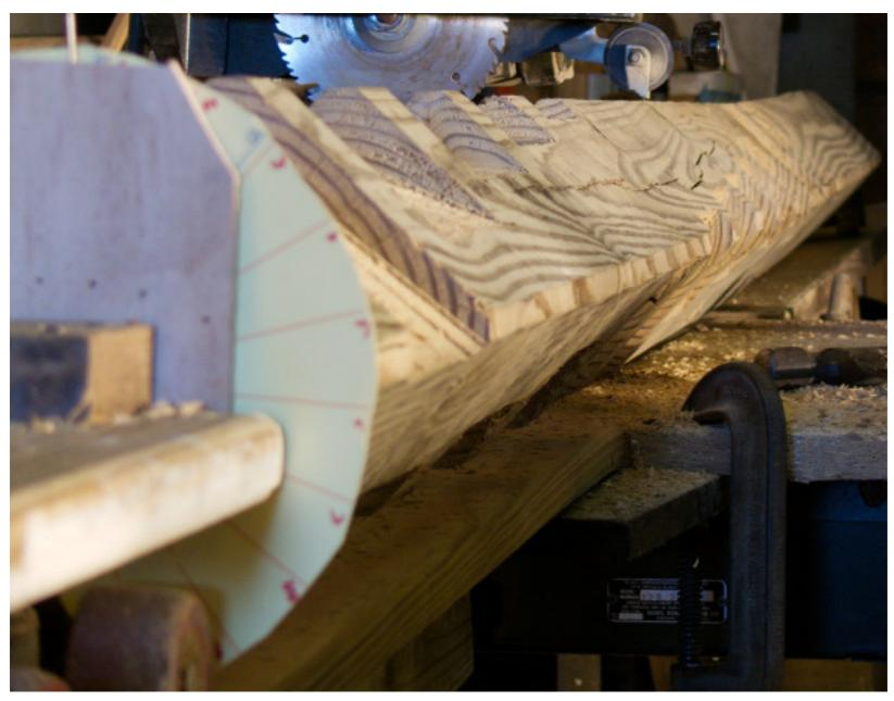
A narrower central core to the column makes for more available step surface towards the center- it's a tradeoff between the strength of the material and the step surface-this design puts a large torsion/wringing force on the wood face at the column where the riser is glued. Each step above the first can rest it's front riser on the back riser of the step below.
